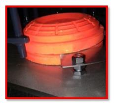
(f) When loading the clays be sure there are no tight spots in the carousel. Occasionally machines can suffer slight damage to the carousel.
